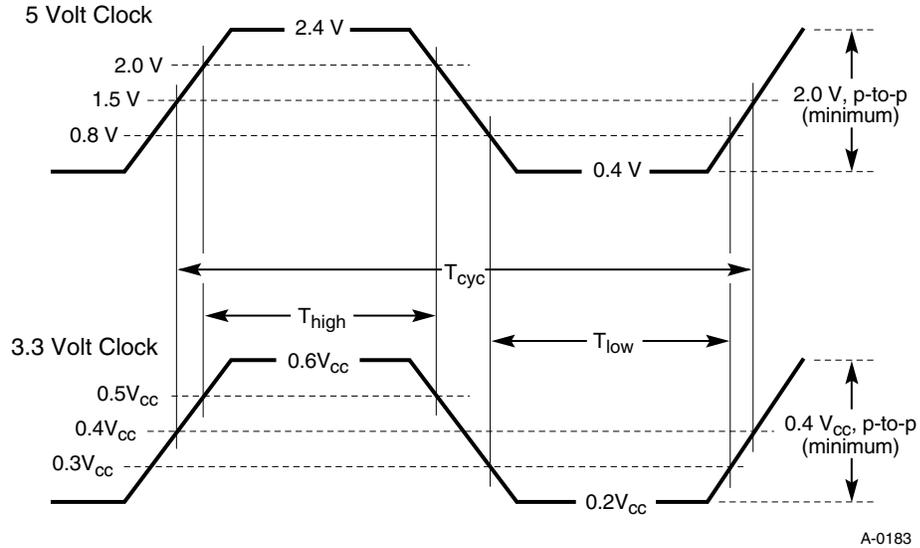
Figure 4-6: Clock Waveforms
