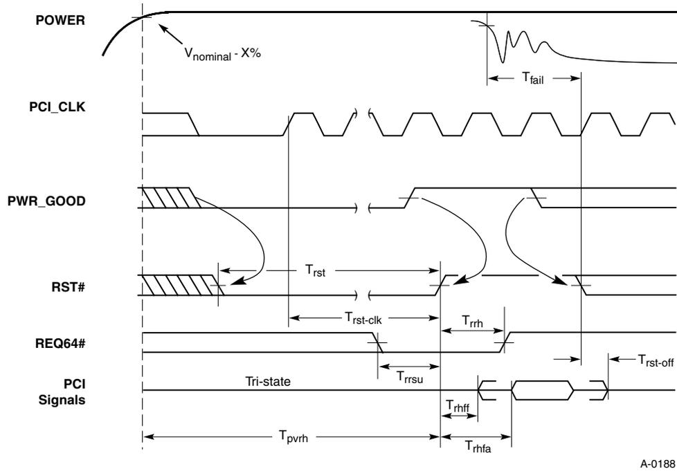
Figure 4-11: Reset Timing <sup>34</sup>
