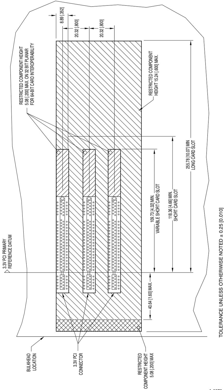
Figure 5-23: PCI Connector Location on System Board
