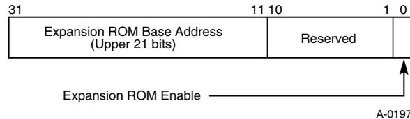
**Figure 6-7: Expansion ROM Base Address Register Layout**
