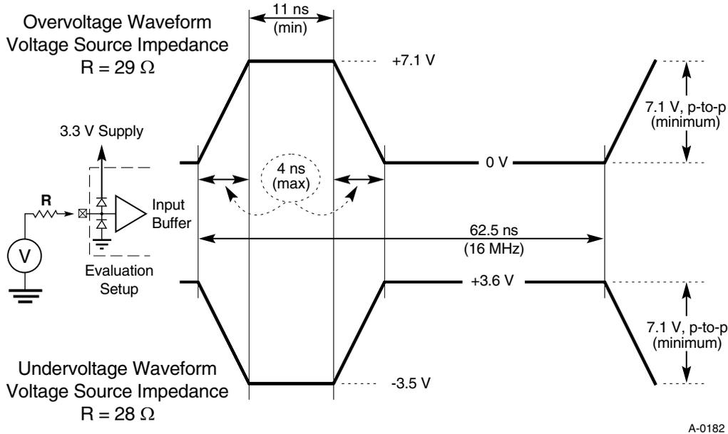
Figure 4-5: Maximum AC Waveforms for 3.3V Signaling
