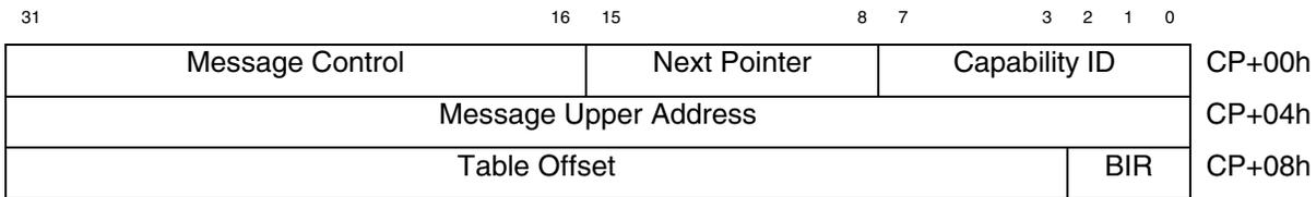
Figure 6-12: MSI-X Capability Structure
